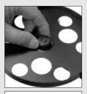
Fig. 18: Place tray onto the mounting bolt hole and thread the attachment knob into place.
